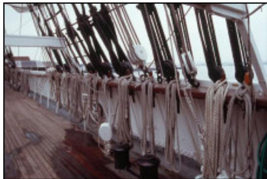
Note the color of the running rigging line compared to the white blocks nearby. Although this is modern material it still shows the effect of weathering on the original color.
