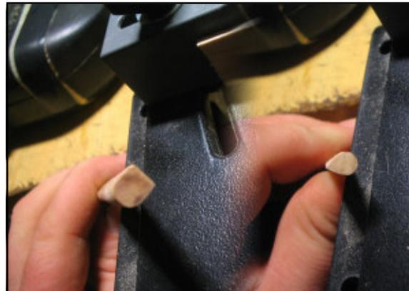
Using bench router table with small round cutter make a groove around new deadeye. Note that router's back fence's hole is covered by extra wooden plank to have proper stopping point. Then sand paper on wooden stock round the edges, cut off the deadeye with fret saw, round other side.
