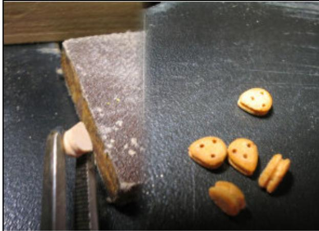
Finally drill three holes and paint ready dead eyes. It took around an hour to produce 10 such deadeyes.
