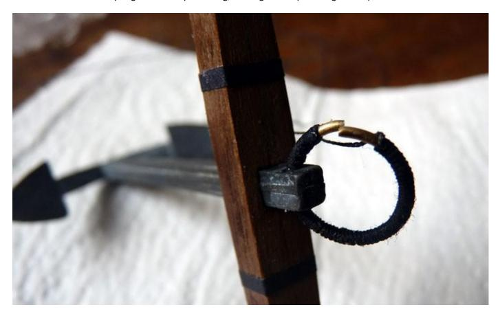
So the ends of the ring were soldered together before serving the remainder of the ring:
