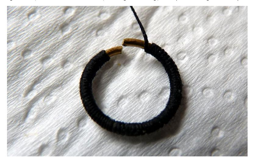
The section of the ring that goes through the anchor should be left bare, so the seizing should be made off at this point and the ring sprung onto the anchor. (I'd suggest blackening the ring before serving it).
