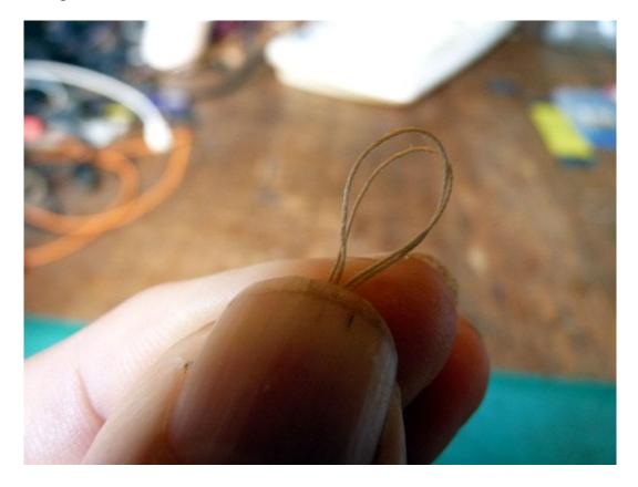
Seize round the base of the double loop you've created. The actual position of the seizing isn't critical.
