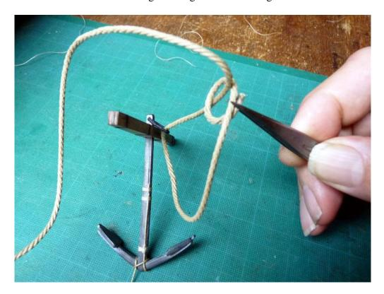
There are three seizings to apply, the first goes, initially, at the point just above the tweezers. Although the loop will be tightened around the cable, the seizing should stay close to the end of the cable; so to start the seizing the cord was passed through one of the cable strands:
