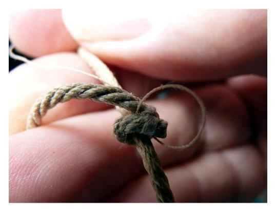
Now for a little bit of cheating! Rather than finishing off the first seizing and starting a new one, bring the cord back under the first seizing and pass it through one of the cable strands just over 1/3 rd of the way round the cable. (As before, keep the lay tight):
