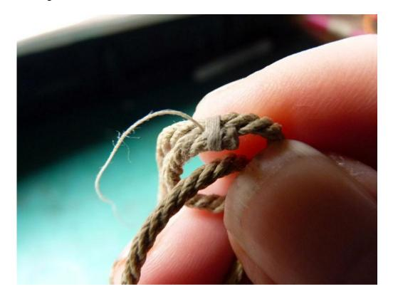
Before making these turns round the centre of the seizing, which will tighten things up considerably, the cable can be pulled through the seizing to tighten the loop around the incoming cable. Take care to keep the lay of the cable tight as you do this:
