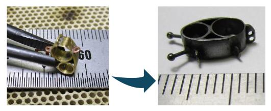
The chemical blackening of metal involves the replacement of a surface skin of base metal with a selenium-based compound (oxidant). There are many types of metal blackening agents; with many generally working on a particular metal to produce a black, green or brown patina. A patina is defined as:
