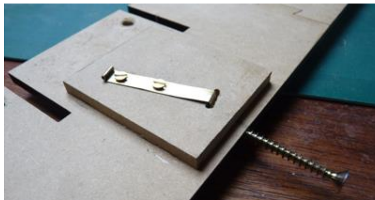
The bronze strip is springy and reaches down to the centre line of the screw hole.
