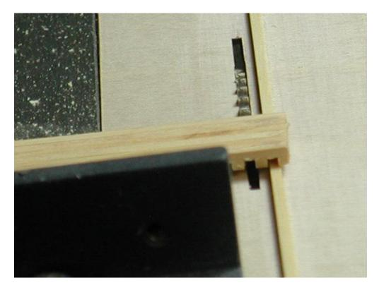
Separate the beams (Acetone will soften the glue and you can run a razor blade down the joints. Be careful – Delicate!)
