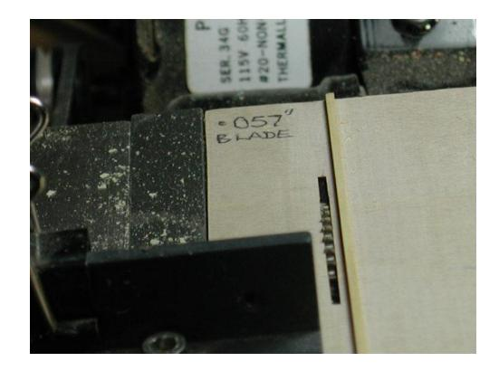
Install the mitre gauge and taking your glued-up block of beams, run them across the saw blade. The blade must be raised to produce a dado whose depth is equal to the thickness of the ledges. For the first cut, the end of the glued up pieces must butt up to the glued on batten thus:
