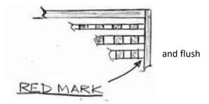
Then glue in the ledges – not too much glue and be careful to not glue the assembly to the jig. It is best if the bottoms of the dados in the beams are slightly above the top surface of the jig.
