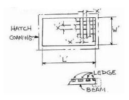
Some thought must be given to scale and the fact that on the real ship dimension 'X' was between 50mm & 70 mm and also the edges of the ends had to finish with a beam or a ledge thus: -
