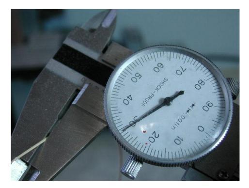
If the dowel is too large, loosen the clamp holding the block and with the sander running, sand a little off the end of the block and try again. Once you have the diameter you want, do not remove the block--you may want more dowel. I always make more parts than I need!
