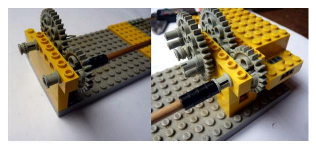
Temporarily lift off the Technics brick at the left-hand end in order to fit the shaft.
