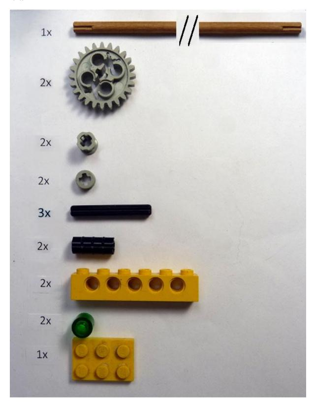
Lego comes in rather clever sizes. As you would expect from a Danish company, the parts are designed to metric sizes and are based on a unit length of 8mm. However, a basic 2 x 4 brick is actually made to an Imperial size! The brick is 1 1/4 inches long, 5/8 of an inch wide and 3/8 of an inch high. That's just under the 32mm x 16mm design dimensions to allow some tolerance when fitting the parts together.
