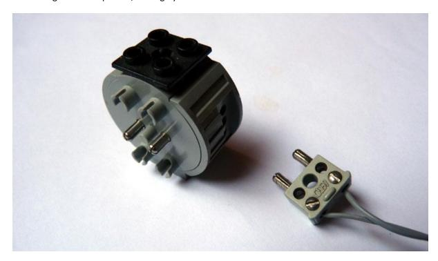
Note: The type of plug shown normally has a centre plastic pin; this has been cut off. This type of plug can be stacked, so it also has a hole between the pins in case the plug you're stacking into it has such a pin.
