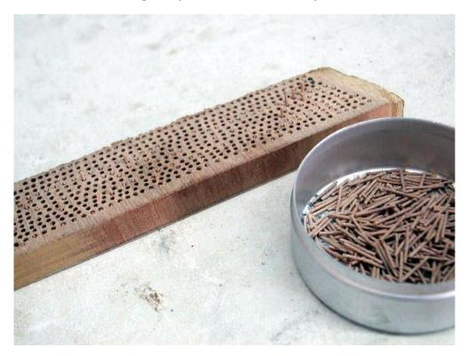
The treenails are best handled with tweezers. Pick one up, dip in glue and insert into holes in planking and frames.
