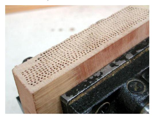
Cross cut a piece slightly LESS than the full length of treenail required. Tap the piece on the bench to dislodge any treenails which may be stuck.
