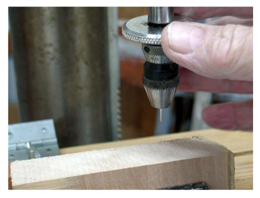
Drill holes until the chuck touches the work piece.
