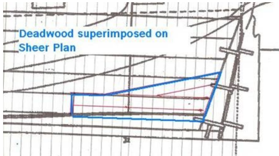
Where frames will contact with deadwood.
