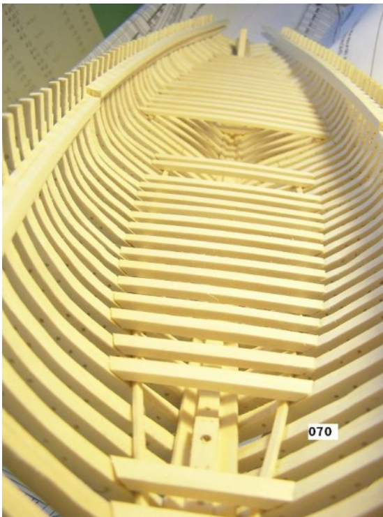
Lower Deck Beams Looking Aft
