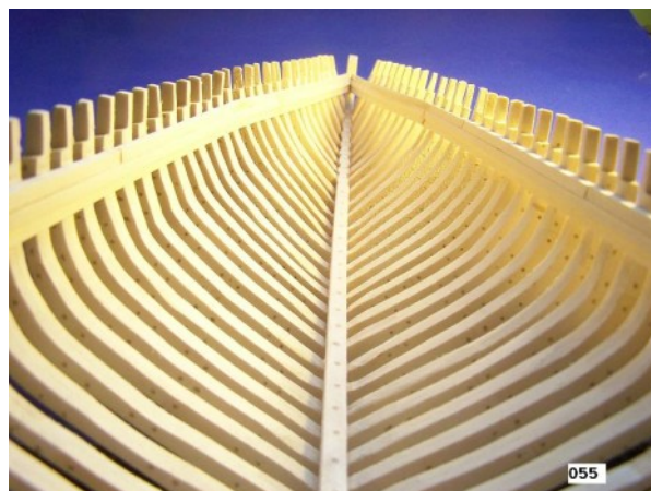
Half Frames at the bow—interior view looking forward
