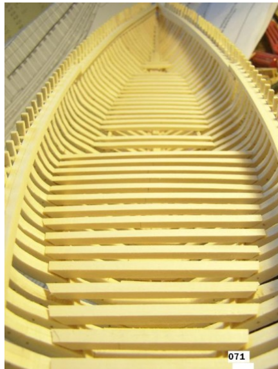
Lower Deck Beams Looking Forward
