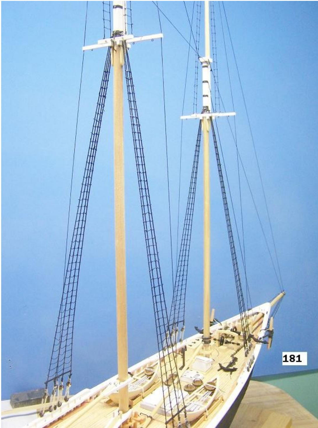
Standing rigging completed – view from the stern
