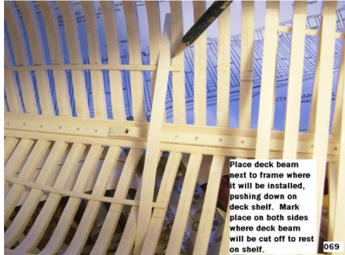
Marking to cut off Deck Beams
