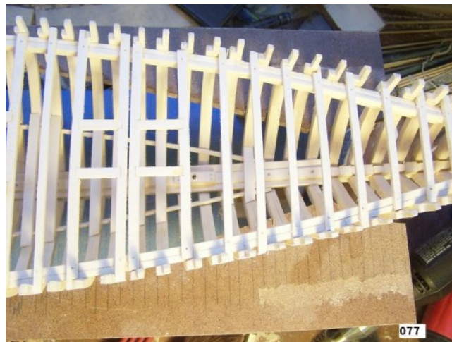
Deck Beams finished—forward section
