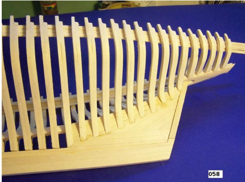
Stern area framing—side view
