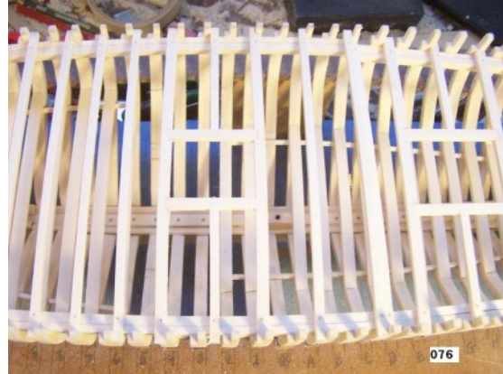
Deck Beams finished—mid-ship section
