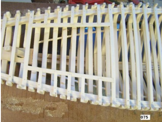
Deck Beams finished—stern section
